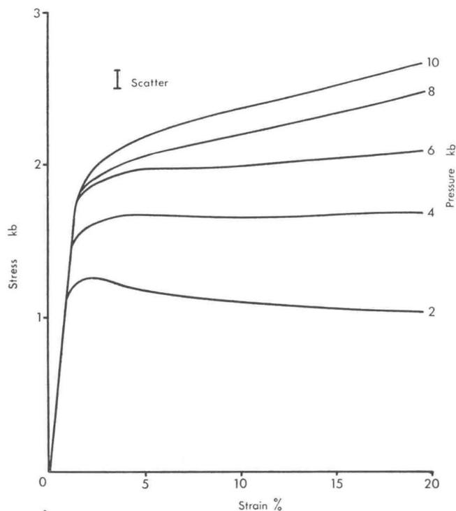
Fig. 1. Stress-strain curves for Three Springs talc at room temperature and confining pressures and shown. The "scatter" band indicates the range of scatter among repeat experiments which applies approximately to all the curves shown
